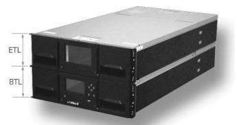
Each module has two removable magazines each with 20 slots for LTO media and five slots per module being used as mail-slots for selective access to LTO media.
