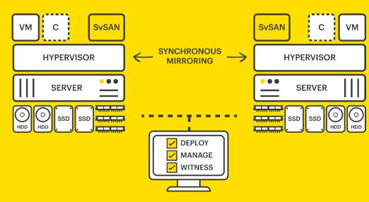
Fig. 1: A typical two-node SvSAN configuration
