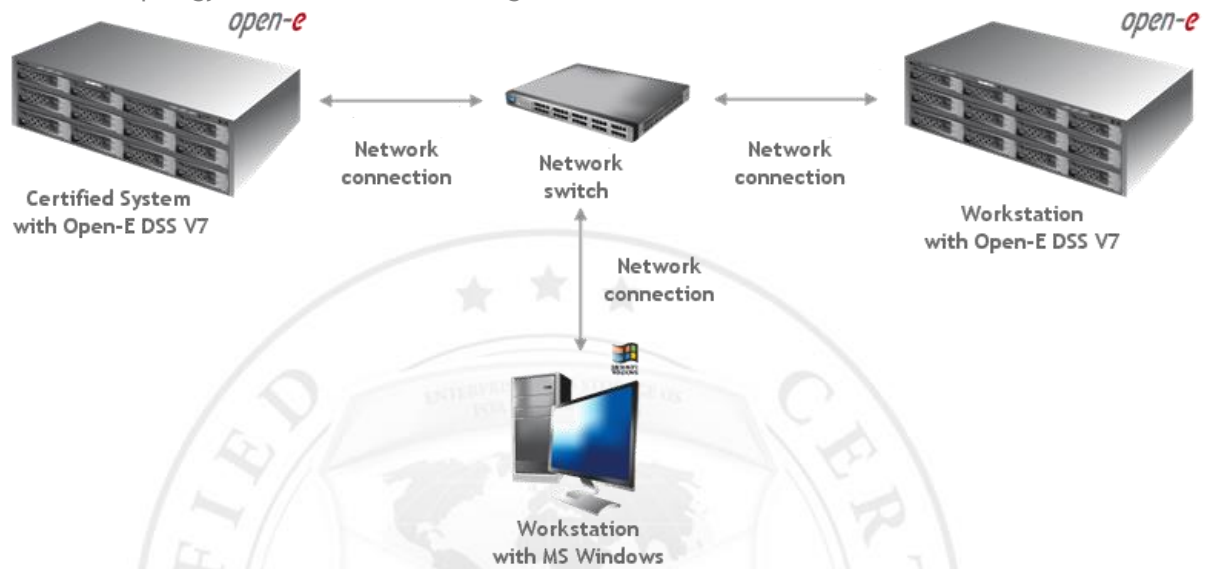
FIGURE 18: Network topology for iSCSI Initiator testing
