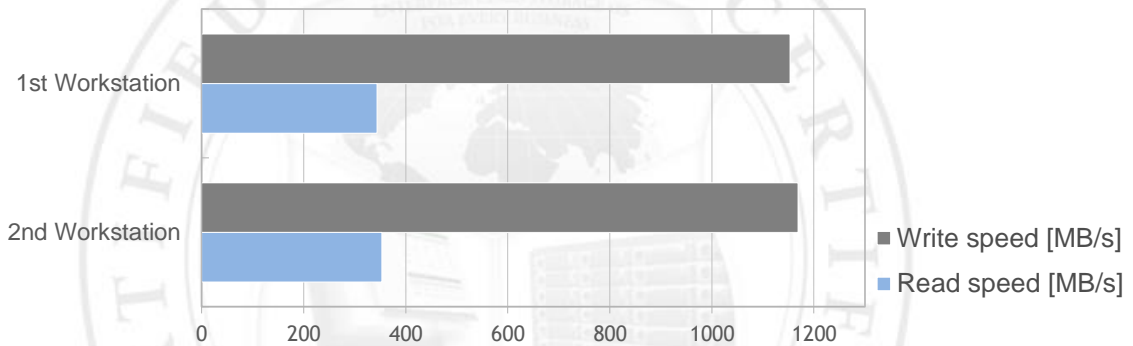
FIGURE 7: Balance-rr bonding mode performance test results chart for QLogic QLE3442-CU
