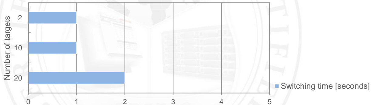
FIGURE 5: Active-Active iSCSI Failover resource groups switching time test chart for QLogic QLE3442-CU (Dual Port 10GbE) with MPIO
