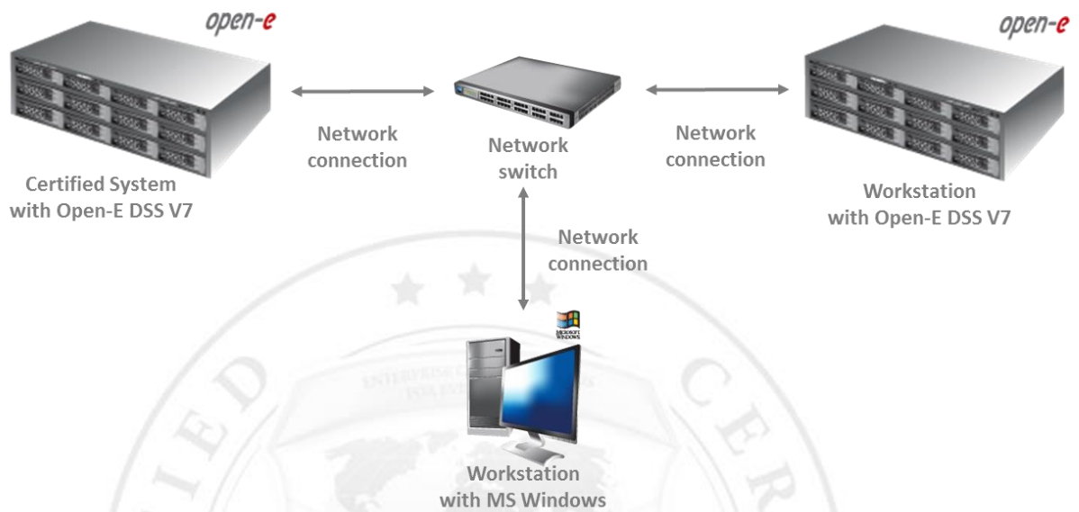
FIGURE 19: Network topology for iSCSI Initiator testing
